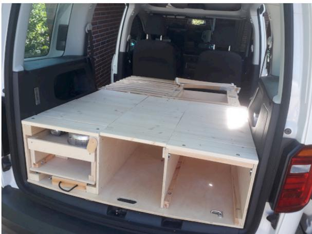
A bottom plate, 113 x 90 cm, (and most other parts) made of 12 mm plywood. Rear of the plate follows the form of the car.
