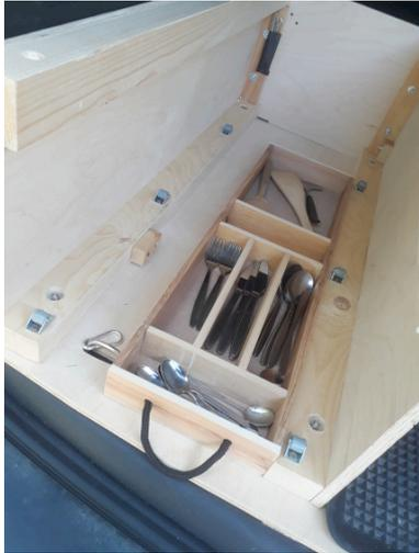
The kitchen drawer is built much the same way, so much narrower than the left side box that there is no friction. It moves on 3 furniture rollers on each side. It also has a roller on the top near the end to support the drawer when it is out. While I had the table saw I also made a cutlery drawer that fits under the kitchen drawer.
